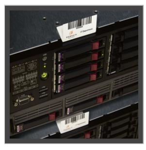
A great alternative to metal mount applications where a standoff will not work, Metalcraft's RFID Server Rack Tag consists of an adhesive label that protects the encapsulated RFID inlay and a non-adhesive, folding tab that offsets the RFID inlay. The label has three sections: a middle section housing the RFID inlay; one end adheres to and provides extra protection for the inlay; while the other end adheres to the asset being tracked.
