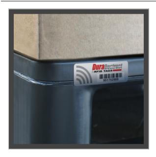
DuraDestruct RFID Security Tag's specialized construction eliminates the transferability of the RFID tag and incorporates two levels of destructibility. If someone attempts to remove the tag the RFID antenna construction breaks into separate pieces making the read range of the tag mere inches. The portion that is still adhered to will literally disintegrate if an attempt is made to remove it from the object.
